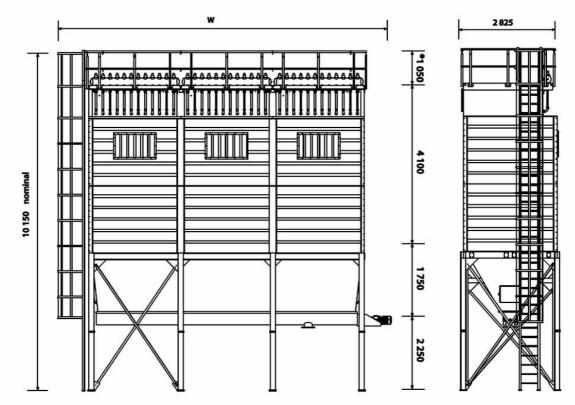
Hopper heights are typical values for 55° valley angle trough hopper \* The Clean Air Chamber height includes toe board
